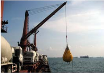
Ship Crane Overload Test
