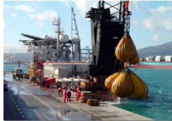
Offshore Crane Overload Test
