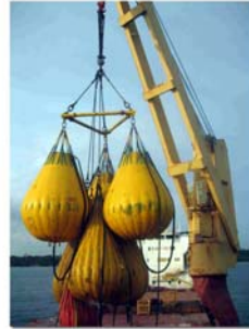
NMF Overload Test
