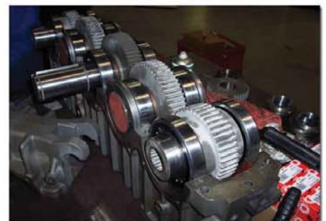
Crane Gearbox Refurbishment
