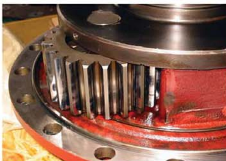
Winch stripdown and rebuilding
